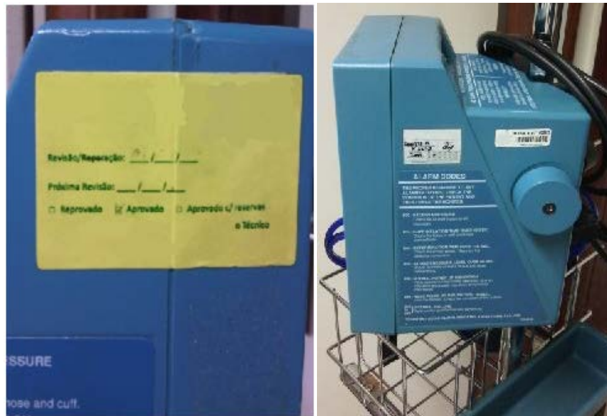
Figure 2: NIBP monitor with its calibration and maintenance labels
